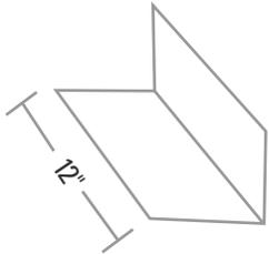
ALWAYS INSTALL INTERLAYMENT UNDER EACH COURSE-STEP FLASHING AND SEAL STEP FLASHING ON TOP OF INTERLAYMENT
